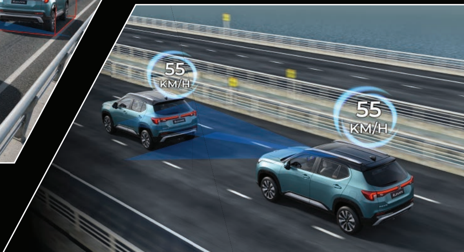
Adaptive Cruise Control with Low Speed Follow™ Accelerates & brakes to maintain a safe distance from other cars while cruising. Low speed follow makes it easier to drive in stop-and-go traffic.
