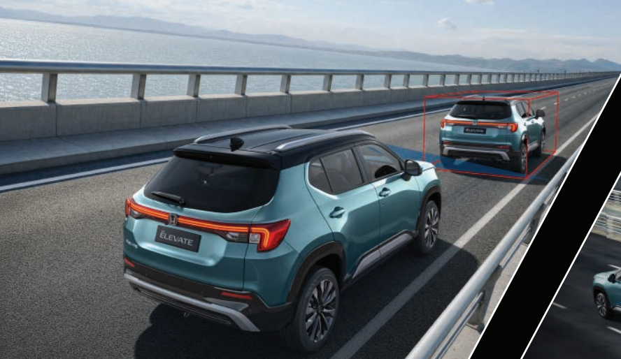
Collision Mitigation Braking System (CMBS) Alerts and applies brakes when a collision risk is detected.
