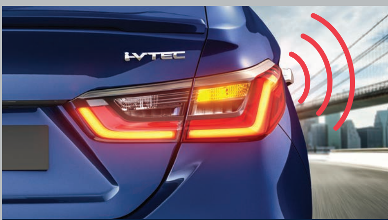
EMERGENCY STOP SIGNAL (ESS)
