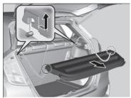
**3.** Disengage the support rods, then remove the luggage area cover.
