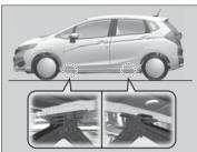
**1.** Place the jack under the jacking point closest to the tyre to be changed.
