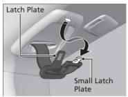
1. Pull out the seat belt's small latch plate and the latch plate from each holding slot in the ceilina.
