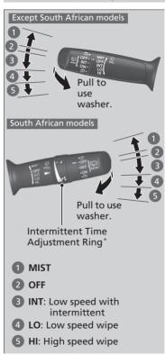
The windscreen wipers and washers can be used when the ignition switch is in ON  $[II]^{*1}$ .
