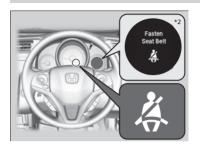
The seat belt system includes an indicator on the instrument panel to remind the driver or a front passenger\* or both to fasten their seat belts.
