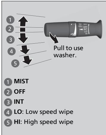
The windscreen wipers and washers can be used when the power mode is in ON.
