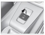
**1.** Make sure the parking brake is applied. The electric parking brake indicator comes on for 30 seconds when you pull up the electric parking brake switch.
