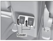
■ Accessory power sockets on the back of the console compartment
