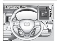
You can adjust the vertical angle of the low beam headlights when the position lights are on.
