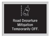
If the system operates several times without detecting driver response, the system beeps to alert you. After that, the Road Departure Mitigation steering assist is temporarily stopped, and the warning sound is given only.
