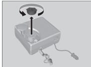
**1.** Take the compressor hose and plug cord out of the back of the air compressor.
