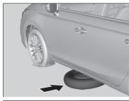
**5.** Place the spare tyre (wheel side up) under the vehicle body, near the tyre that needs to be replaced.
