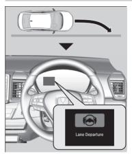
The front camera behind the rearview mirror monitors left and right lane markings (in white or yellow). If your vehicle is getting too close to detected lane markings without a turn signal activated, the system, in addition to a visual alert, applies steering torque and alerts you with rapid vibrations on the steering wheel, to help you remain within the detected lane.
