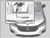
**3.** Pull up the bonnet latch lever (located under the front edge of the bonnet to the centre) and raise the bonnet. Once you have raised the bonnet slightly, you can release the lever.
