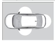
When you carry the keyless remote, you can lock/unlock the doors and open the boot.
