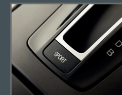
SPORT MODE The Sport Mode provides a more engaging driving experience by adding more battery assist to the propulsion motor for increased acceleration.
