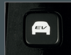
EV MODE EV button lets the driver select purely electric operation and in this mode a green EV icon gets lit on the instrument panel.
