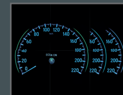
ECO ASSIST The Eco Assist system has illuminated arcs on the side of speedometer to show if the vehicle is being driven in an efficient style. The color changes gradually in response to the overall driving style.
